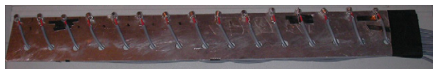
Fig. 2. A photograph of the in-duct microphone array. Fifteen 7 mm electret microphones were mounted on a thin 50 mm × 400 mm aluminium plate. The microphones were positioned at the edge of the plate, with the centre of the capsules 25 mm apart.
